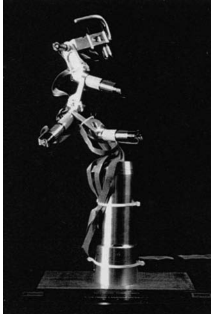
FIGURE 4.31. DIESTRO, a six-axis isotropic manipulator.
